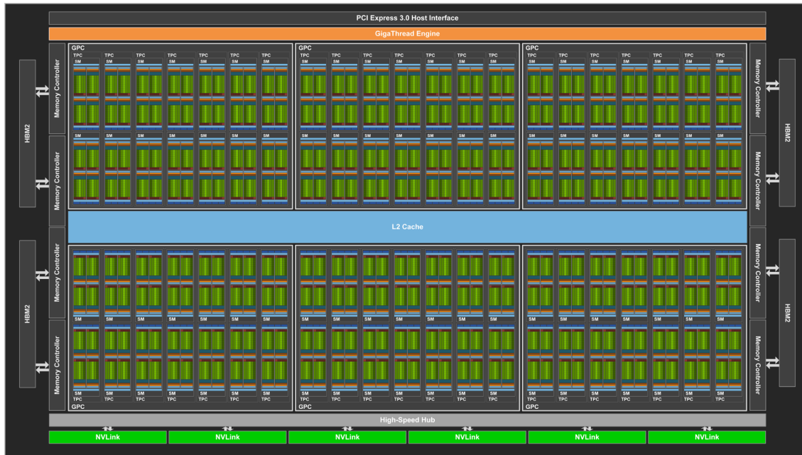
Figure 2.2: NVIDIA Tesla V100 architecture [2]
