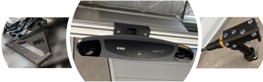
Figure 3: Pallet-mounted marker (left), NDI Polaris Vega® XT optical tracker (middle), tool-mounted passive markers (right).
