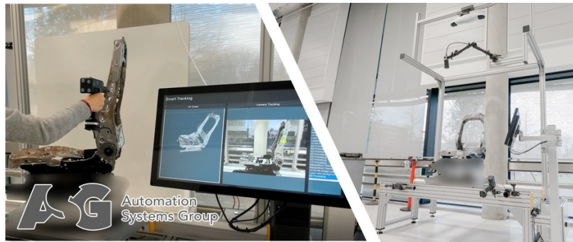
Figure 4: Screen-based work instructions with 3D model view (left) and overview of the DAMPO station set-up (right).
