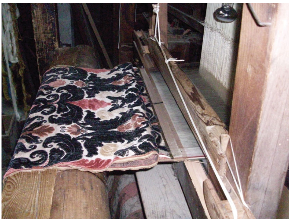
Figure 4. Production of silken velvet using an eighteenth-century European loom. Manifattura Bevilacqua, Venice, 2009. In Europe, textile design was created through the medium of weaving and the setting up of looms was a long and costly procedure. Photo by the author.
