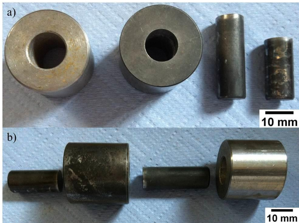
Figure 4.1: Steel die and punch set used to prepare pellets (a) Top view and (b) side view arrangement in order of application
