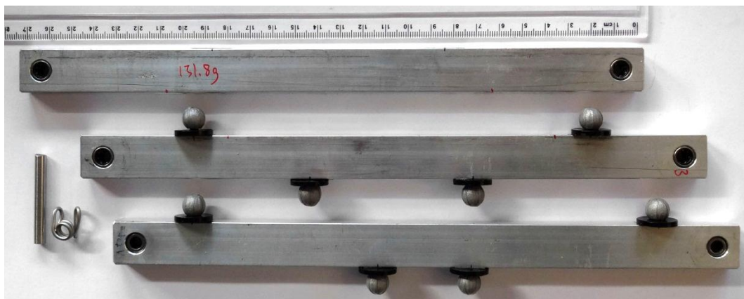
Figure 4.2. Three pendulum segments and one of the silver steel axle and one axle retaining spring shown at the bottom left. Segments are aluminium with needle bearings press fitted into each end. All segment have identical dimensions. The bottom two segments are shown with motion capture markers attached, which were used for tracking the positions and orientations of the pendulum during measurements.
