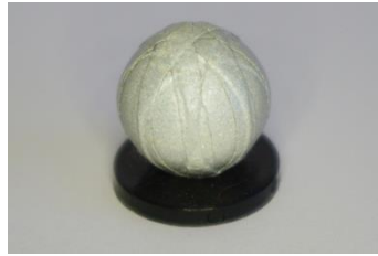
Figure 3.3. A motion capture marker. A plastic sphere covered in high visibility tape, connected to a black plastic base, providing a flat surface at the bottom to be attached to the subjects using double sided tape. This marker has a diameter of 14mm; the base has a diameter of 16mm and thickness of 2.5mm.
