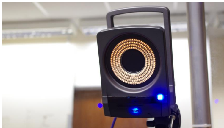
Figure 3.2. A Vicon MX infra-red camera used for motion capture. It has a 4 row red/infra-red ring light providing the infra-red light providing the light source for the infra-red camera. at the centre of the ring light is a infra-red pass filter, placed in front of the lens and camera sensor. At the bottom right of the camera is a blue indicator light.
