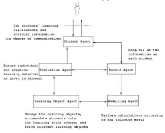
Figure 3. System Architecture
