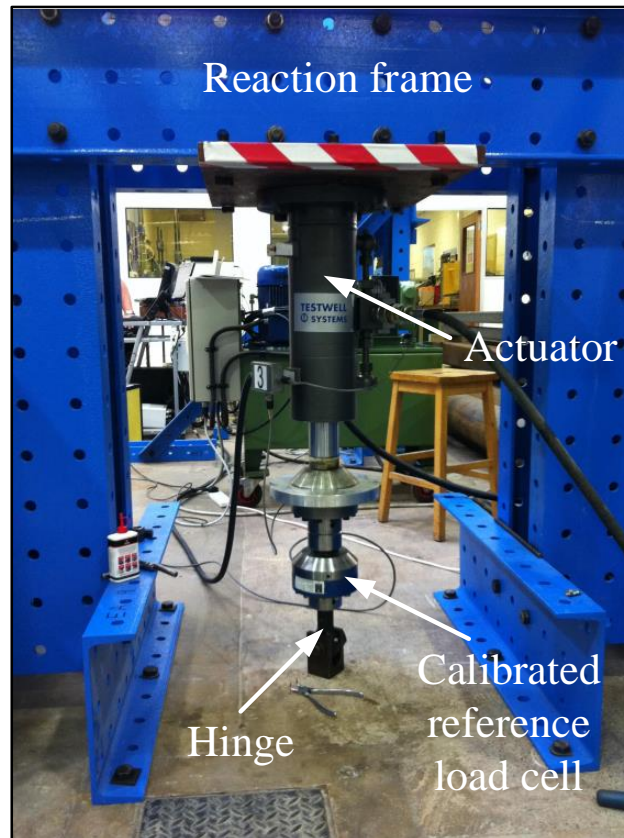
Figure 5.26: Calibration of the actuator load cell in tension
