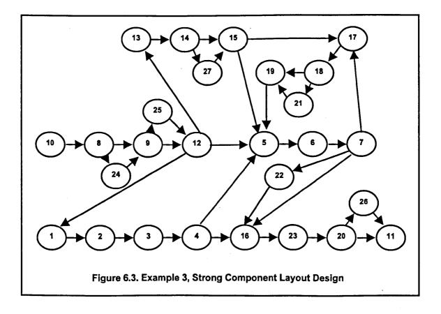
The Strong Component approach suggests a network-based layout design as shown in Figure 6.3
