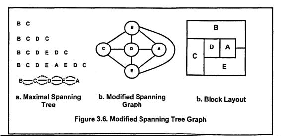
A proposed computational variant of this method, which constructs character strings from the spanning tree, is shown in Figure 3.6.a; following the dotted lines it would be BCDEAEDC. A computational implementation of these procedures using character strings was presented by Carrie et al (Carrie A.S., Moore J.M., Roczniak M., Seppänen J.J., 1978).
