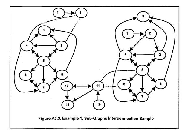
The sub-graphs obtained from the previous steps (Steps 4.a, 4.b and 4.c in Figure 5.3) are linked using the list of unused arcs (Step 4.d in Figure 5.3), which are the in-between links (Steps 4.a.iv, 4.b.iv and 4.c.iv in Figure 5.3). It should be noted that the sub-graphs obtained represent manufacturing sub-systems or modules, which might be interrelated, but some trial and error should be expected in order to obtain the best possible facility locations.
