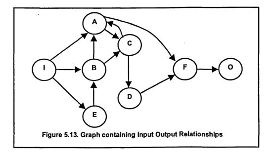
Figure 5.13 shows the relevance of considering the location of input and output ports when developing a layout design. The comparison between this figure and Figure 5.10 suggests that neglecting these ports may lead to inappropriate layout designs.
