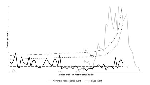
Figure 6. The measured outcomes for a main component, showing signs of maintenance induced failures.
