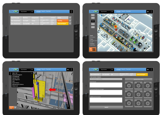
Fig. 13. vueOne fault tracker mobile application's main screens.
