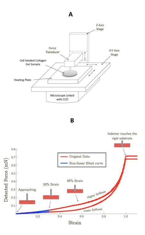
**Fig 1**. (A) The schematic setup of bio-nano-indentation tester. (B) Typical loading force-displacement curves of collagen gels with higher and lower stiffness indented by a flat punch.
