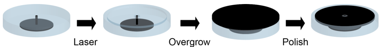
Figure 8.2: Schematic of the proposed method for all diamond ring-UME growth. Step 2, producing the ring.
