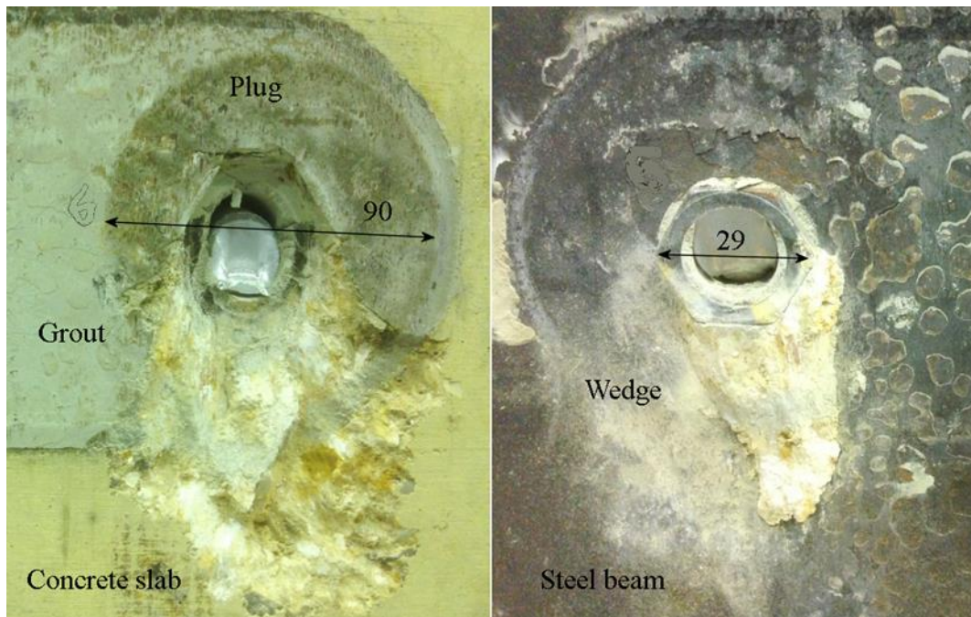
Fig. 5.17. LNSC Concrete wedge failure in pushout Test 6
