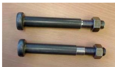
Fig. 2.11. New connectors machined from studs (Lam and Saveri 2012)
