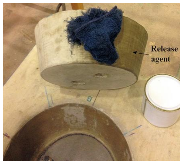
Fig. 4.24. Applying the release agent to concrete plug and slab pocket
