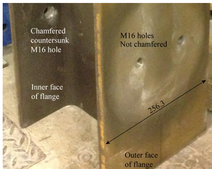
Fig. 4.38. Chamfer countersunk seat in FBSC Test
