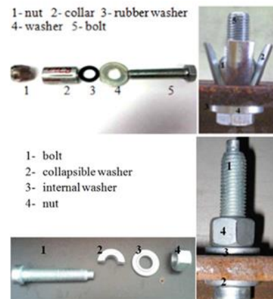
Fig. 2.9. Two types of blind bolts (Pathirana et. al. 2016a)
