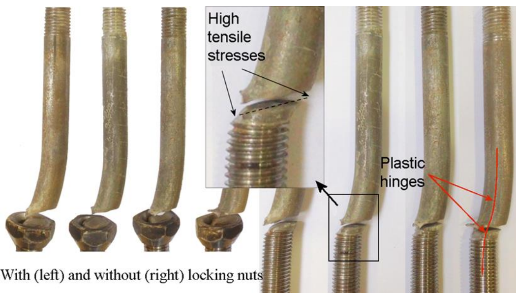
Fig. 5.16. Bolts deflected shape of LNSC pushout Test 6
