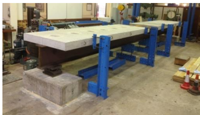
Fig. 4.52. Lateral supports for concrete slab during construction
