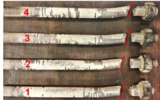
Fig. 6.8. Deflected shape of bolts of FBSC Test 3
