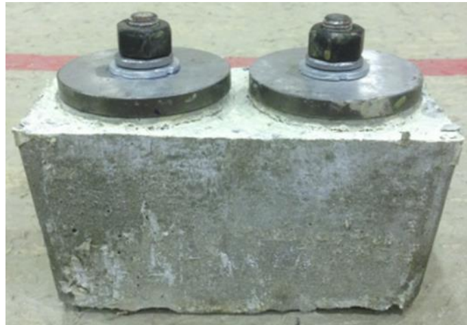
Fig. 5.13. Pulled out slab pocket after LNSC Test 5
