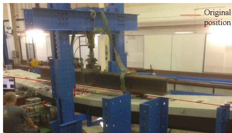
Fig. 7.4. The deflected shape of the composite beam
