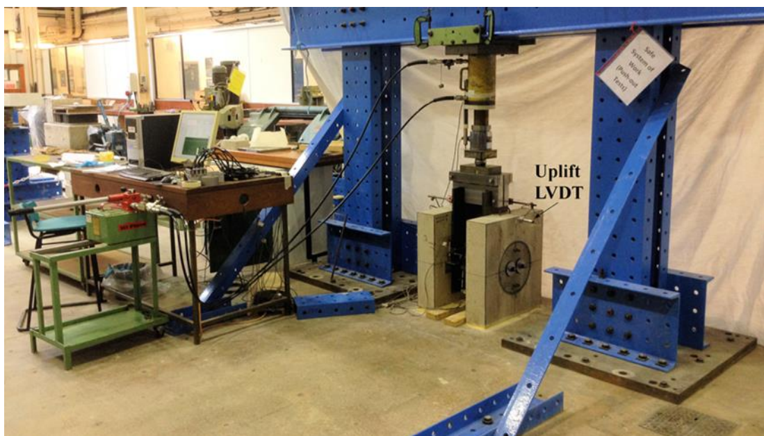
Fig. 4.17. Overview of testing rig and specimen for LNSC pushout tests 3
