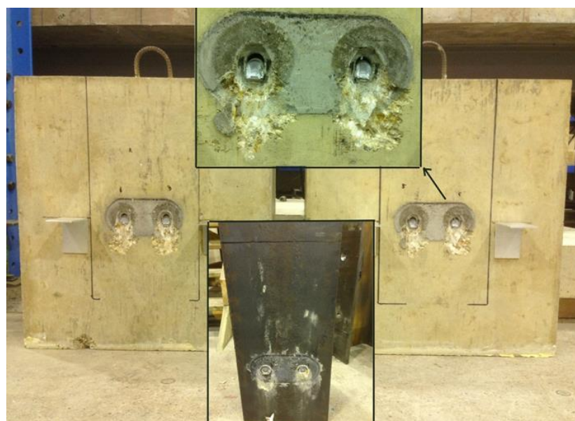
Fig. 5.26. Concrete wedges after push-out Test 6
