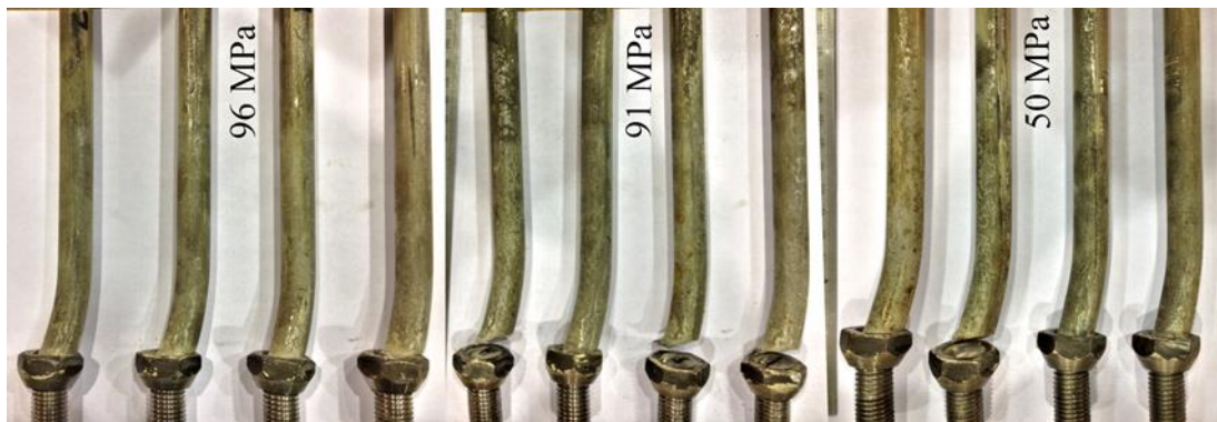
Fig. 5.37. Deflected shapes of M16 bolts for different plug concrete strengths
