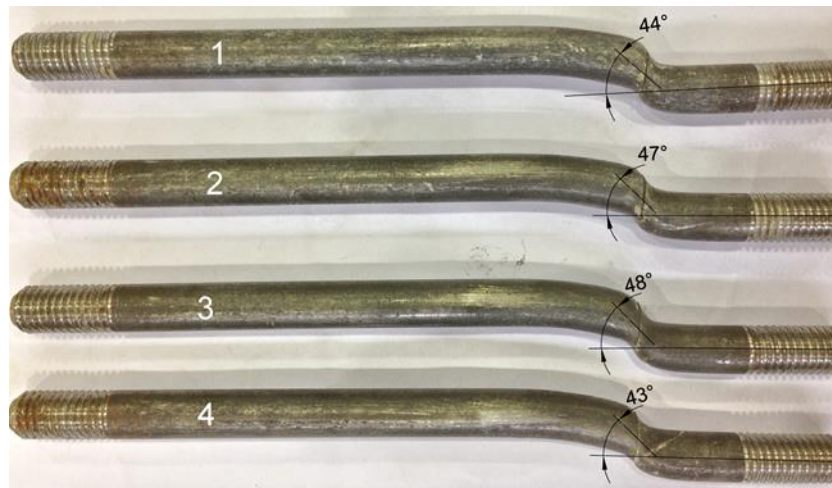
Fig. 6.36. Bolts deflected shapes of FBSC Test 8
