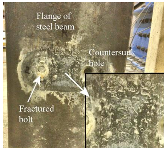
Fig. 6.32. Irregularity at the flange of FBSC Test 11
