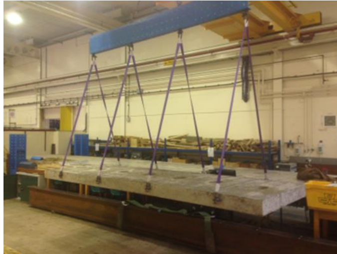
Fig. 4.54. Lifting of one concrete panel
