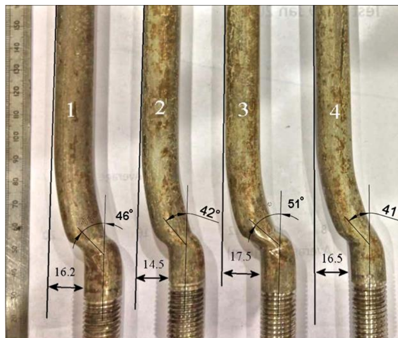
Fig. 6.23. Deflected shapes of bolts for FBSC Test 6
