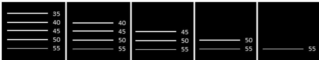
Figure 4.11. Exposure pattern progression used for the building of 1 mm-high walls. Each 100 \mu\text{m} resin layer was exposed to all 5 projections sequentially, with the pattern progressing every 5 seconds.
