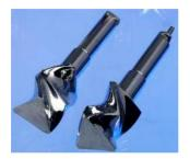
Figure 3. Roller rotors employed in the batch mixer.
