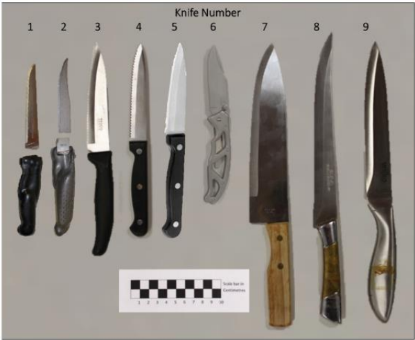
Fig. 4. From left to right, Knives 1-4 serrated, 5-9 plain edged. Five Confiscated knives donated by the Physical Protection Group of the Metropolitan Police (Knives 1-2 & 6-8), and two knives (Knives 3 & 9) used in experiment 2. One knife (Knife 5) used solely in experiment 1 along with Knife 5.
