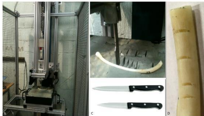
Fig. 6. A) Drop Test Rig; B) Knife marking dry rib; C) Two knives used in experiment 1, Knife 4, left and Knife 5 right; and D) 4 cut marks generated by Knife 4
