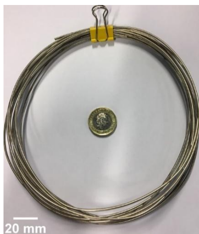
Figure 14. Photograph of a 5 m 1.27 mm ID Pt/SiO 2 coated tube reactor along with a pound coin for scale.
