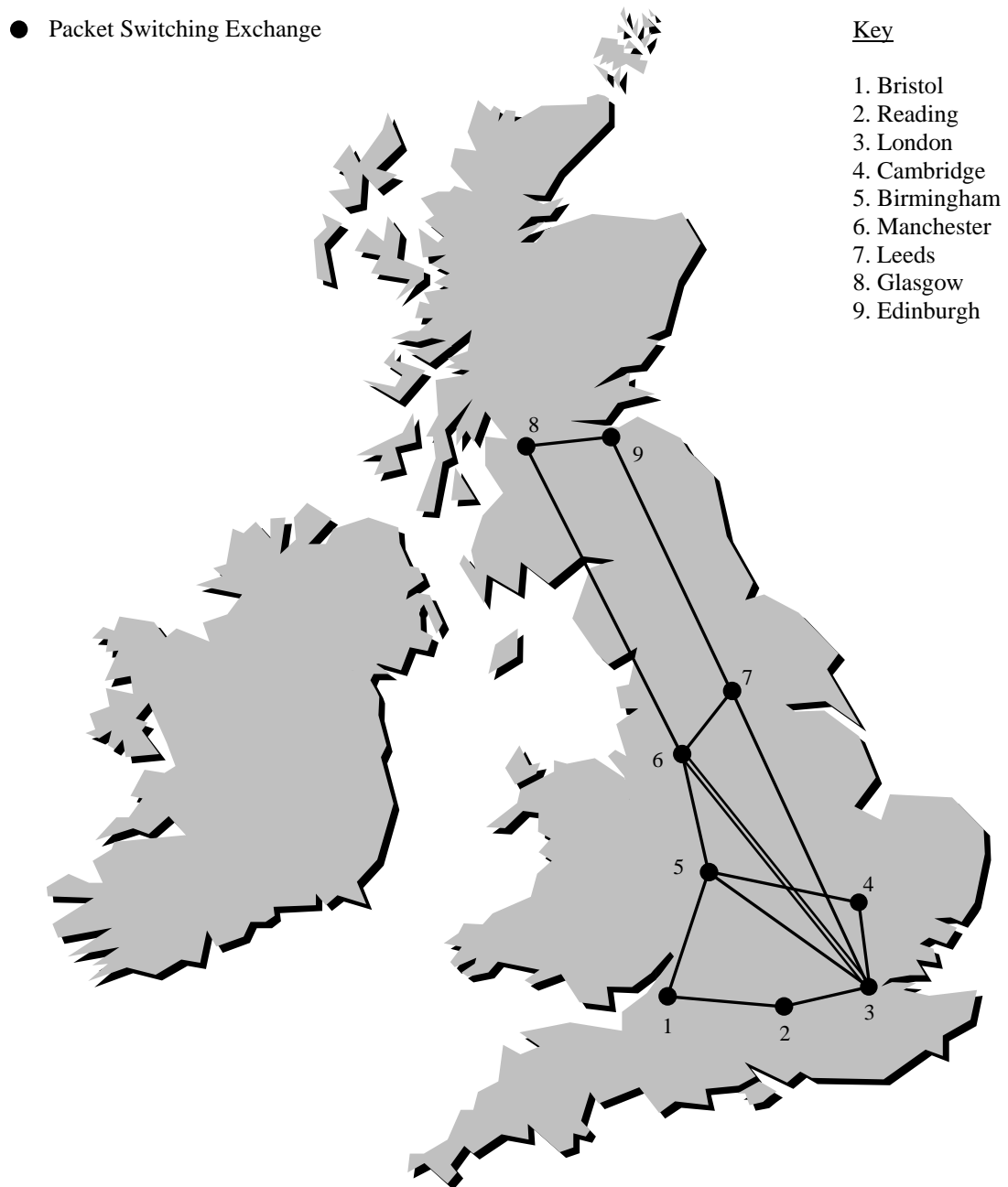
Figure 5.2. The Packet Switching Service network in 1980. 32
