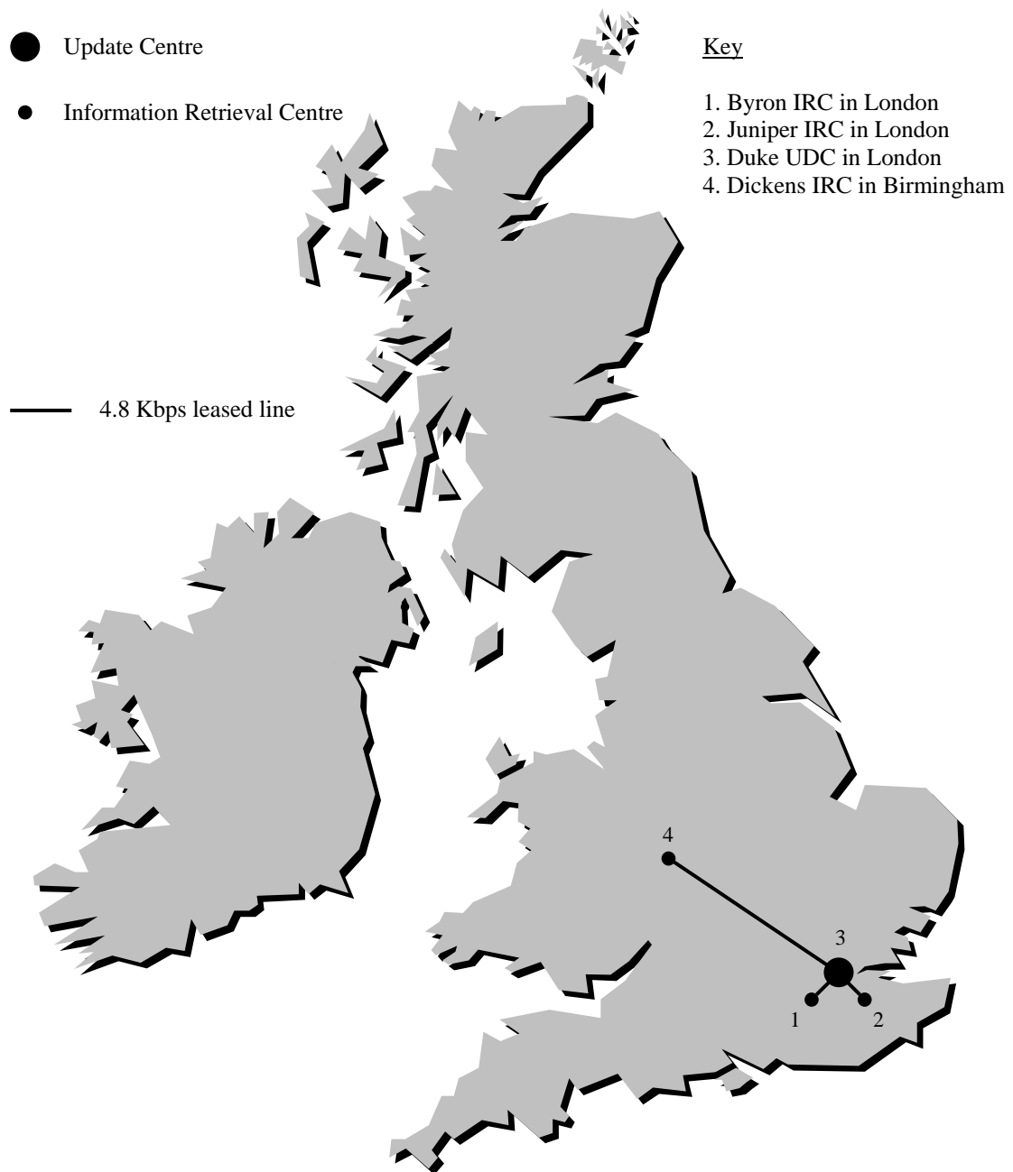
Figure 4.1. The Prestel network in September 1979.
