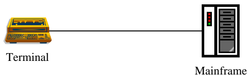
Figure G.1. A point-to-point connection.
