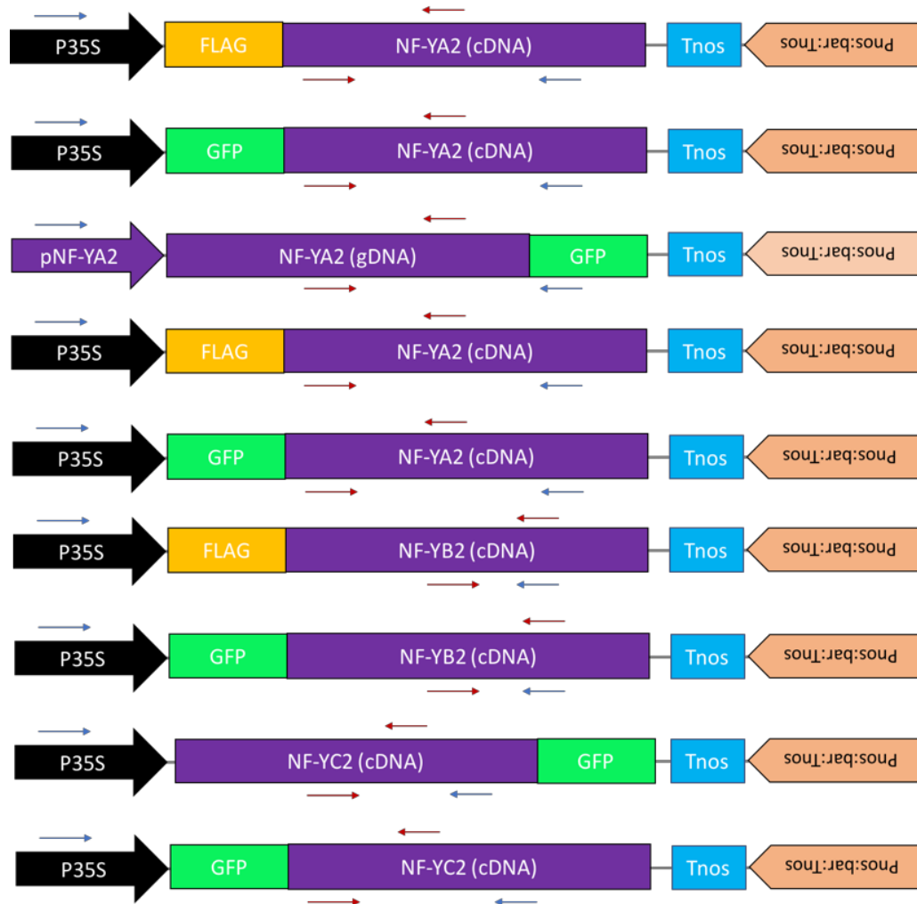
Figure 3.1 – Schematic representation of all gene constructs generated. Red arrows indicate position of primer pair used for q-PCR, while blue arrows indicate primers used for genotyping.
