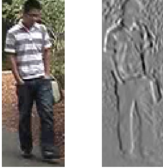
Figure 2.2: An example of the 3 \times 3 filter in Figure 2.1 applied to an image. It can be observed that the filter highlights vertical edges within the image. In CNNs, the weights of the filter are learned by backpropagation.
