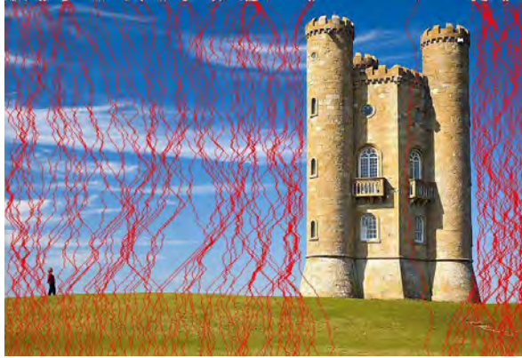
Figure 2.3: An example image showing how seams are found within an image. The red seams run vertically through the image, mostly running through the flat background which contains less information.
