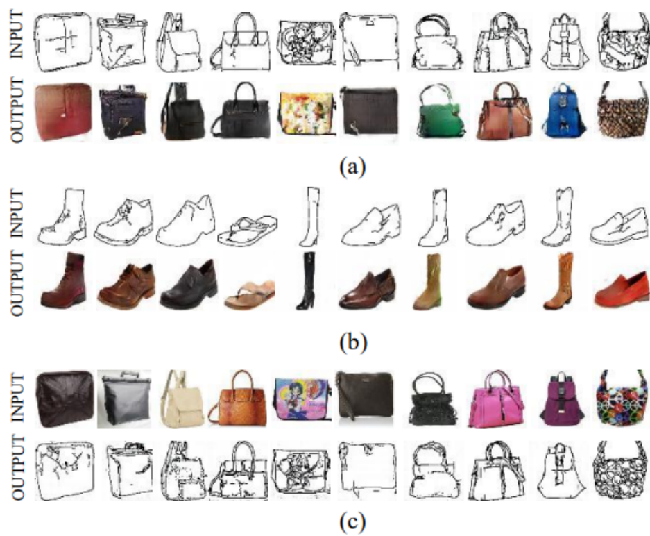
Figure 1.24: The samples from GAN that Learns to Discover Relations Between Different Domains (DiscoGAN) [100]. a) The colored images of handbags are generated from the sketches of handbags; b) The colored images of shoes are generated from the sketches of shoes; c) the sketches of handbags are generated from the colored images of handbags
