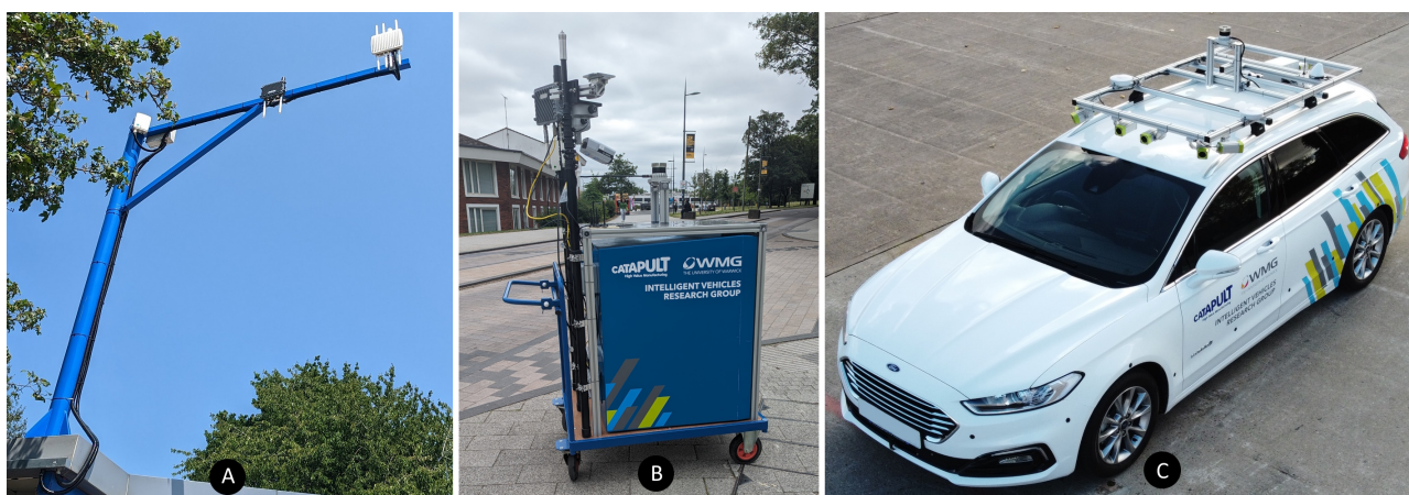
Figure 5. The University of Warwick campus is used as a testbed for V2X and vehicle research and has (A) fixed V2I equipment and RSUs, (B) mobile V2I equipment and RSUs, and (C) research vehicles equipped with V2I equipment, vision systems, and OBUs. The images (by the authors) are of WMG V2I equipment.
