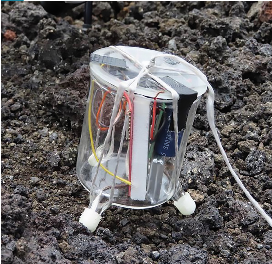
Figure 16: An off-grid sensor payload deployed via Unmanned Aerial Vehicle (UAV) for the remote monitoring of radiation levels around Chernobyl. Image credit: Interface Analysis Centre, University of Bristol.
