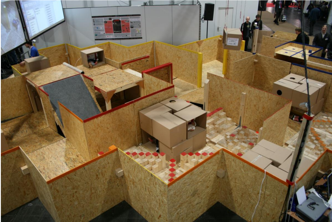
Figure 1 - Test course used in 2008 German open competition. To the top of the picture, the yellow autonomous area can be seen; at the center and bottom the red area can be seen, including full cubic step fields and a 45° ramp; to the lower right, two orange half-cubic step fields can be seen; to the upper right, the blue pick and place area can be seen. No radio drop-out zone was present at this competition.
