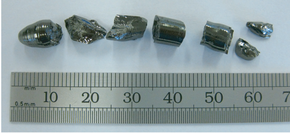
Figure 3.1: Pieces of a grown boule of TbMnO 3 , which broke upon removal from the image furnace.
