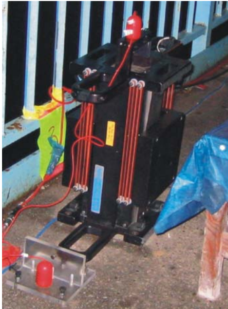
Figure 6: Electrodynamic shaker operating in the vertical mode.
