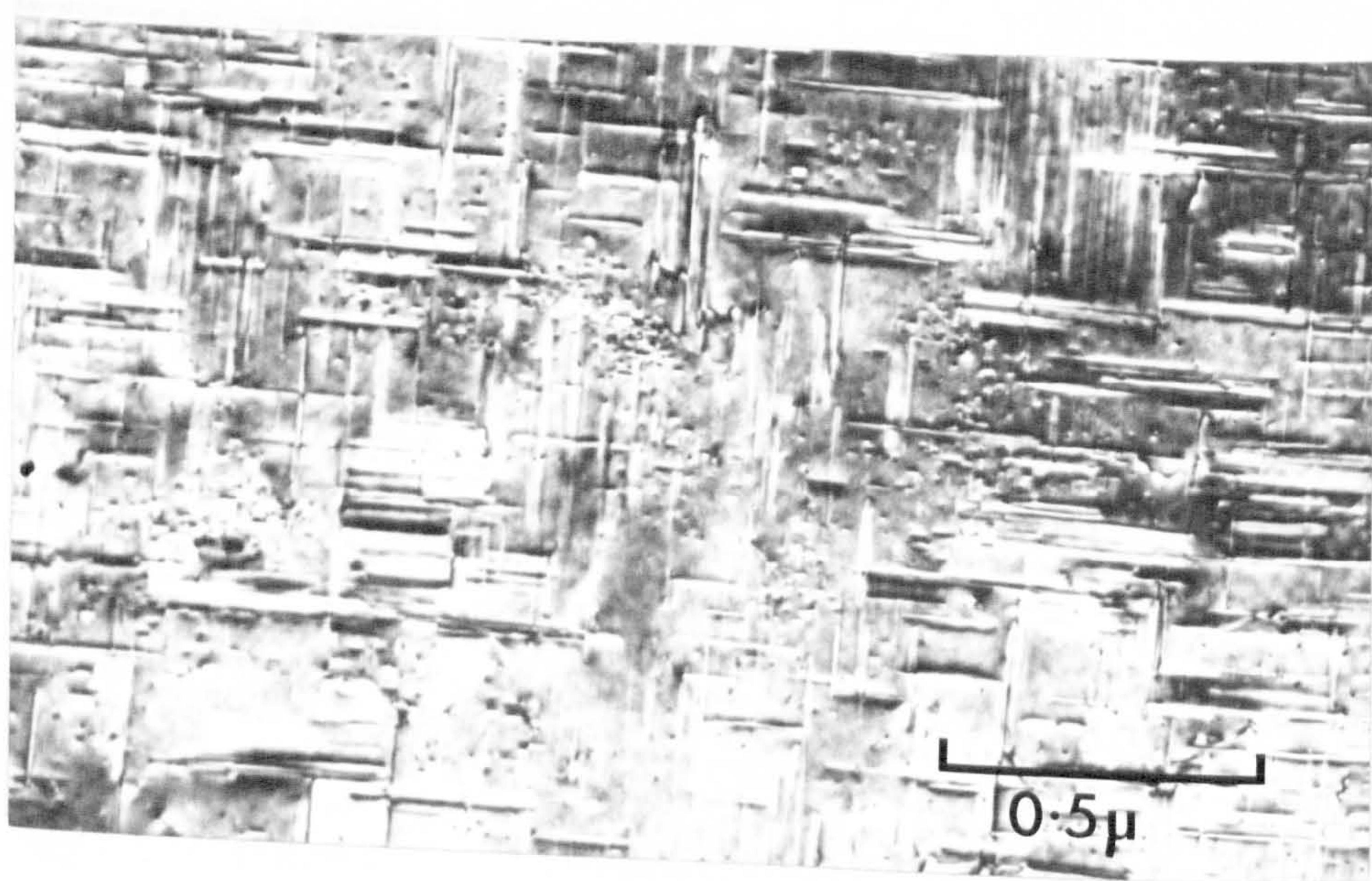
Figure 5.9 Al-1.2% Mg_2Si : The effect of the heat treatment illustrated by Figure 5.8 on the precipitate microstructure. (c) 3 minutes at 250^{\circ}C without any further ageing; (d) as for (c) plus 24 hours at 160^{\circ}C .
