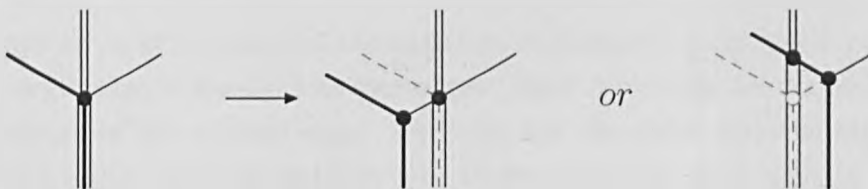
Figure 3.10: Moving a real vertex v of degree greater than 3 when the cycle goes along one single edge and one group of edges.
