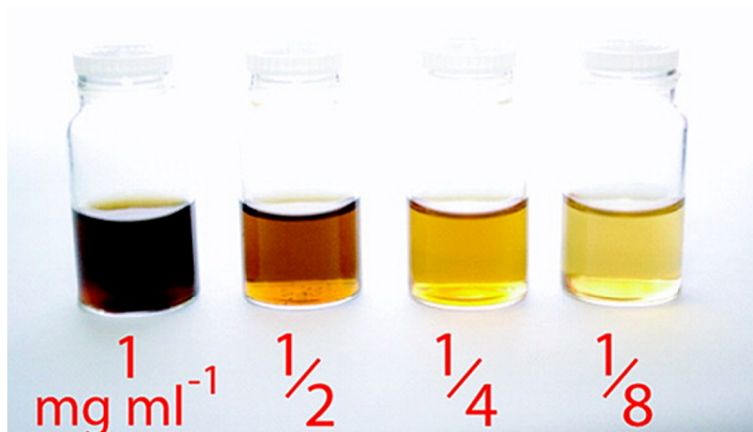
Figure 2.2 Aqueous dispersions of GO of concentrations 1, 1/2, 1/4, and 1/8, \text{mg ml}^{-1} from left to right.
