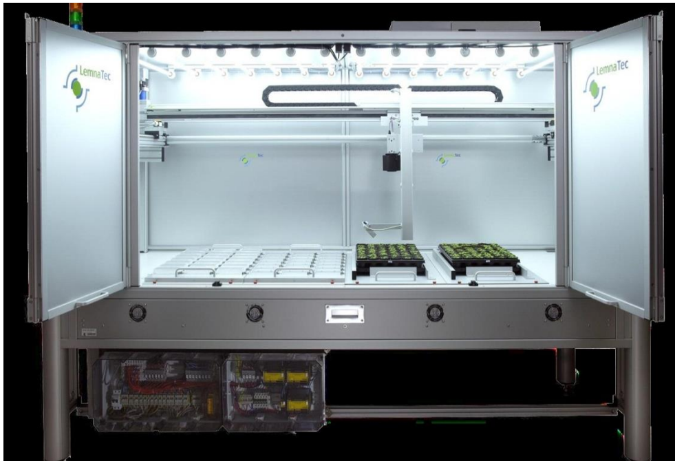
Figure 1-2: Scanalyzer HTS developed by LemnaTec to study plant phenotyping in simulated environments. Image Credit: [11].
