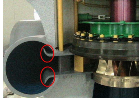
Figure 23 Guide-plate (circled) shown on the model of turbine
