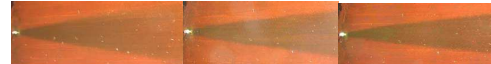
Figure 22 SSLC results for the turbulent wedge under zero, mild and strong (favourite) pressure gradients respectively [8].
