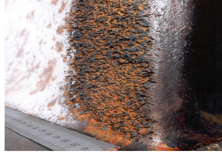
Figure 11 Typical sponge-like erosion pattern caused by a leading-edge cavitation attack (4000 hour operation) [18]
