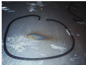
Figure 6 Heated sign on the top surface between guide vanes
