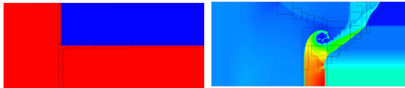
(a) \rho and finest level patches at t = 0 . (b) \rho and finest level patches at t = 2.5 .
