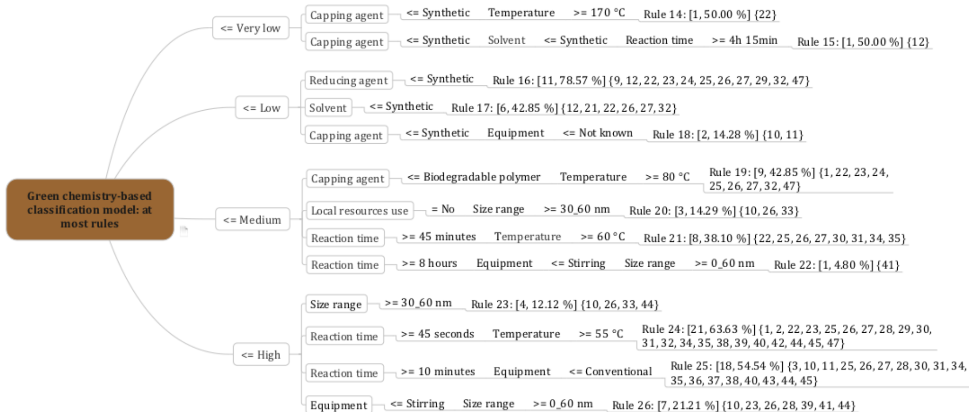
Figure 6-3: Green chemistry-based classification model - At most rules. Each rule is reported as follows: Rule x: [y, z] {p, q, t} with: x = rule number; y = number of protocols that support the rule; z = coverage factor of the rule (i.e. percentage of number of protocols that satisfy the conditions and are assigned to the class or union of classes); p, q, t = identification numbers of the protocols in the dataset
