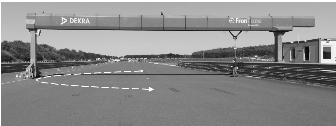
Fig. 2.3.: Rotatable bridge system.
