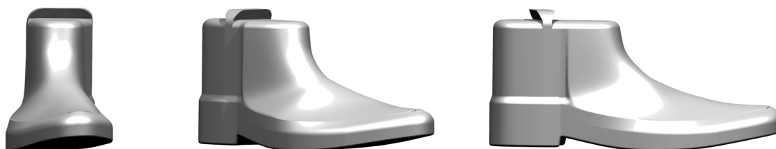
Fig. 5.5.: Right foot model of the 10D Pedestrian Dummy Device a) front perspective, b) 45° perspective, c) 90° perspective.
