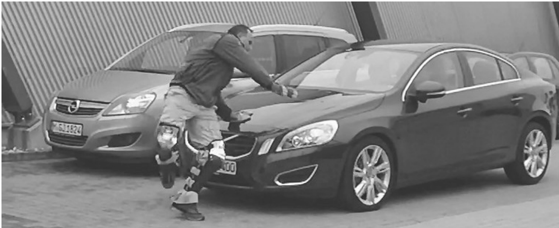
Fig. 2.2.: Pedestrian detection system with emergency braking tested by the ADAC with a stuntman, photo: ADAC e.V. [37].
