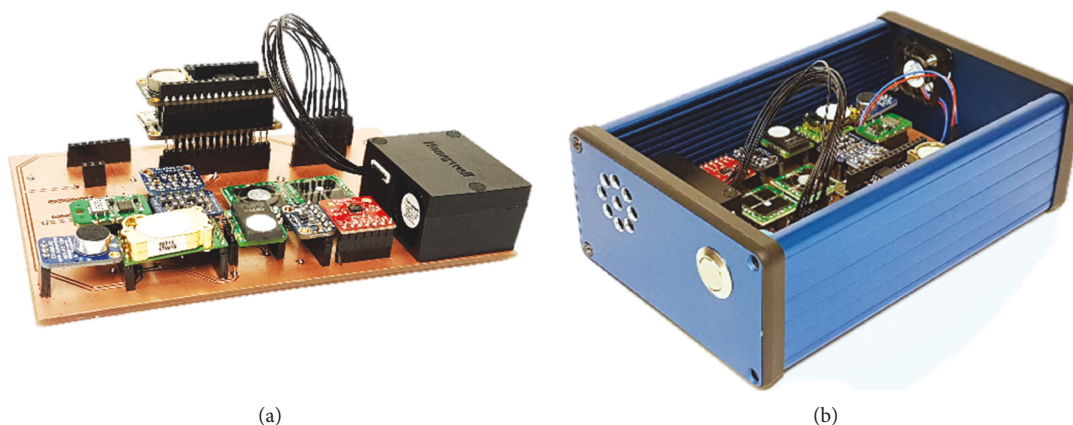
FIGURE 2: IEQ-monitoring device assembly stages: (a) sensor modules mounted on a custom PCB and (b) assembled prototype with internal connections.
