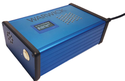
FIGURE 8: Fully assembled IEQ-monitoring device.
